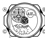
Correct indicator disk position
